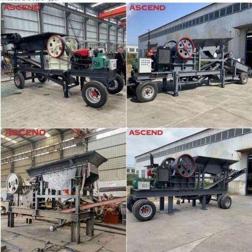
The mobile crushing station can directly enter the site for processing, which reduces the transportation of materials and saves the transportation cost of raw materials. It can be considered as a combination of feeding, crushing, and screening machines in stationary crusher plants.
