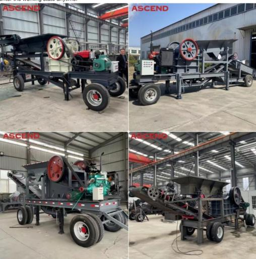
Diesel mobile jaw crusher is widely used for crushing various materials like stone, granite, trap rock, coke, coal, manganese ore, iron ore, emery, fused aluminum, oxide, fused calcium carbide, lime stone, quartzite, alloys, etc. The application of tires makes the machine more convenient to move and adapt to various application, especially when your place lack of electricity or you need to move machines frequently.
