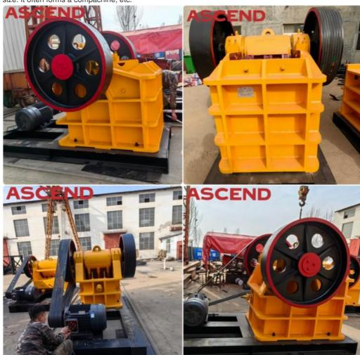
It is applied to fine crushing of various material of which compressive strength is less than or equal to 320Mpa, is applied to relatively small feeding material granularity and relatively small discharging gate, and is fitted for the secondary crushing. Hongji provides a complete line of stone production; the output is widely used in road, bridge, house, high building, railway highway, water project as the type of construction material, such as aggregate, foundation stone, etc.
