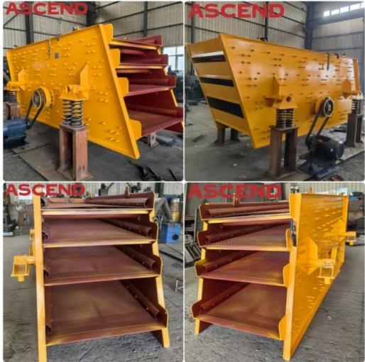
It can be featured with 2 layers, 3 layers, 4 layers. It is used to sort and classify the materials accoding to the particle size by its circular vibration.
